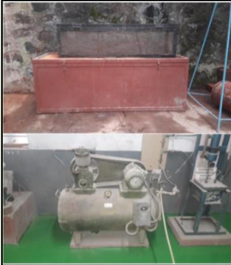
**Mr Sandip G. Sawant has developed Cyclic Loading Equipment for Testing of RCC Beam which was being used for his own research and further can be used for consultancy and student projects.**
